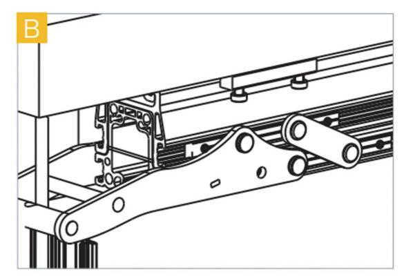
For doorframes up to 6.5m in length, additional lever force is applied
