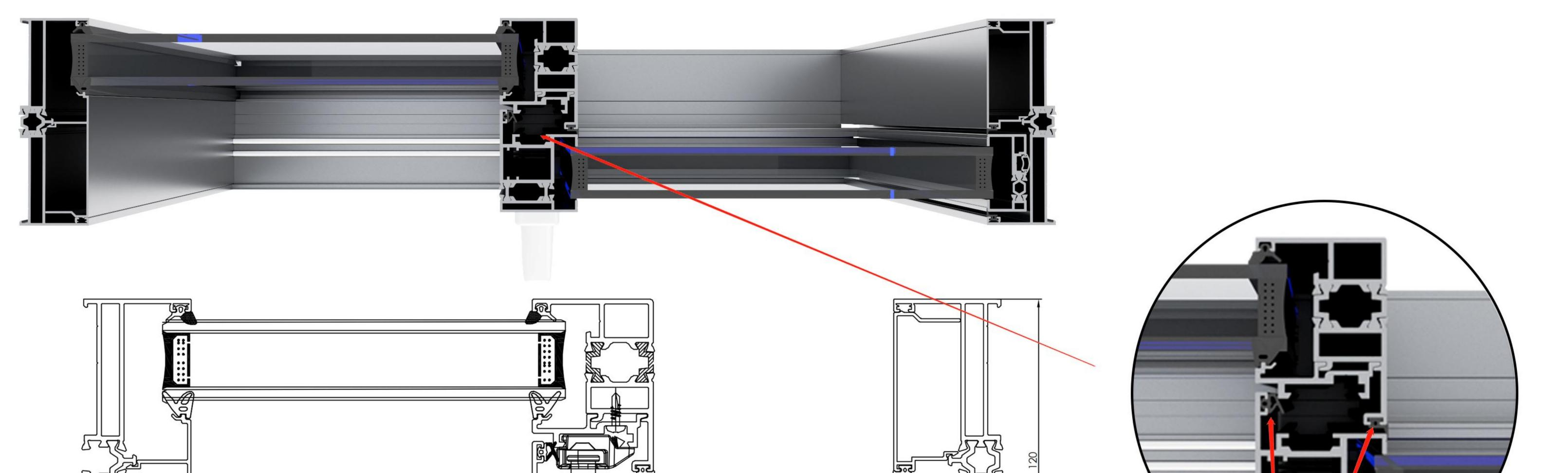
The locking system is located in the middle frame of the window sash, when properly installed, can provide good airtightness and weather resistance.
